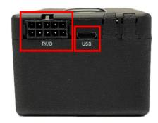
**USB:** Micro-USB port is reserved for FW upgrading (USB cable is not included into the kit).
