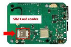
Attention: Remove SIM PIN code before using.
